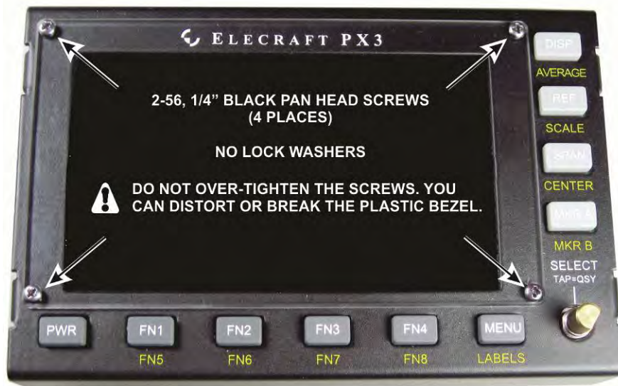
Figure 30. Front Panel PC Board and Bezel Mounted on Front Panel.
