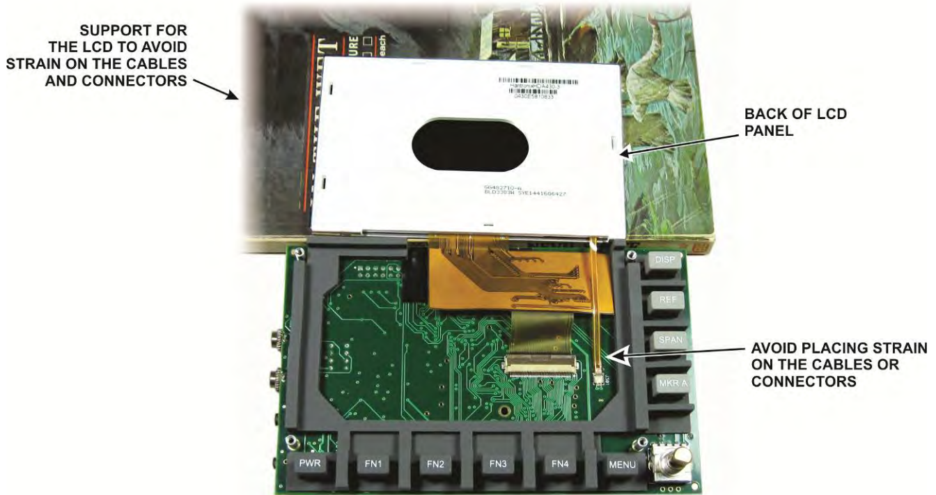
Figure 44. Removing LCD Panel from Rubber Key Matrix.
